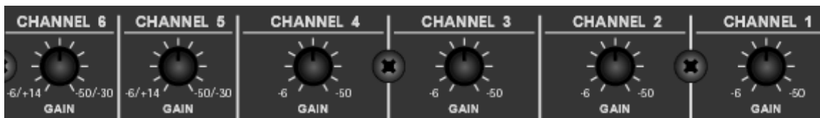
[ Acceptable input sensitivity per each channels ]
