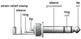
For connection of balanced and unbalanced plugs, ring and sleeve have to be bridged at the stereo plug.
